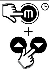
While continuing to hold down the , press the and keys at the same time. The display shows "AL" (alignment) for 2 seconds and then the actual alignment value (the default value is 0).
