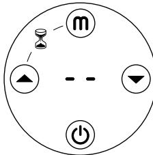
When the product is turned on, it activates in Automatic mode. The message "AU" is shown for 3 seconds on the display and, after, the set temperature is shown:
