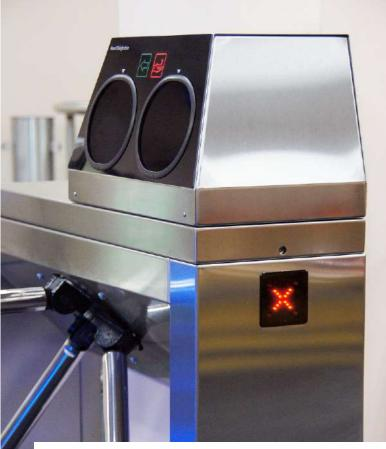
An automatic hand disinfection sprays a sanitizer when a person places their hands in the disinfection unit. In the lower part of the turnstile body there is a 5 liter tank with sanitizer liquid. The sanitizer liquid is extracted from the reservoir by vacuum pumps and sprayed onto the hand from several points. The disinfecting unit is made of stainless steel.
